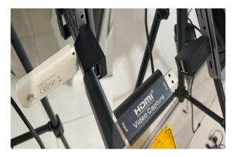
6a. If you have a USB hub or splitter, plug this in and then plug the HDMI capture card and 4G dongle into this.
