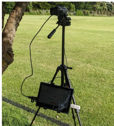
A MAS kit composed of: Chromebook mounted on a tripod, camcorder with capture card, and 4G connectivity USB.
